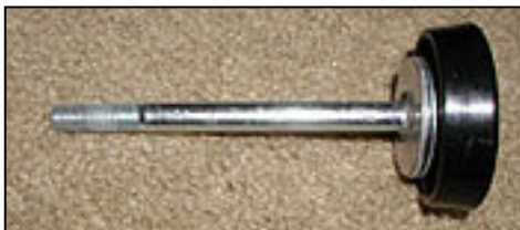
Close-up of the clamping bolt. It's a 5" long 3/8" bolt with three large fender washers and a retainer to hold everything together.
