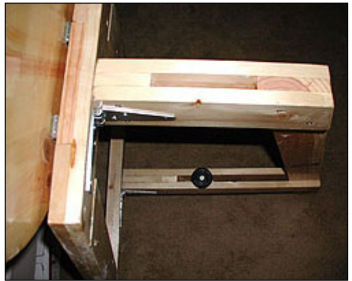
Another view of the top of the legs where the clamping bolt goes through and attaches to the top. The clamping bolt (black circle at bottom) is stored in the bottom of the legs with another T-Nut. In retrospect it could have also been used to keep the leg from 'flopping' when folded up if placed horizontally.
