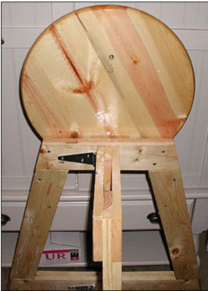
Top up with the folding leg open. The clamping bolt goes through the opening in the top of the leg and into the hole on the underside of the top where it threads into a T-Nut.
