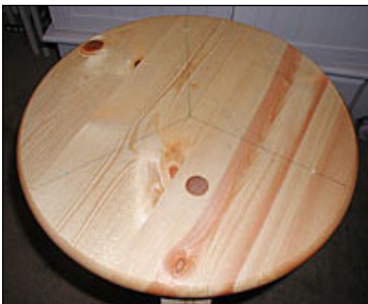
The top of the top. Notice the plug where the T-Nut was inserted. The lines are for placing screw holes for cleats and make it easier to relocate the holes and avoid the plug.
