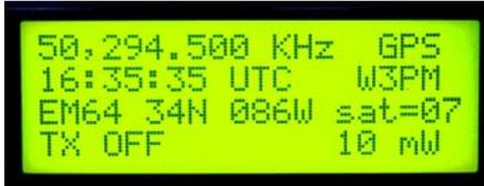
The transmitter may be put into a standby mode by depressing the Transmit Inhibit pushbutton. Depress again for normal operation. The GPS or WWVB receiver will remain on for time updates during standby periods.
