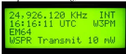
The internal time clock may be used to synchronize transmission times over a period of a few hours. The time must first be manually set to an accurate time source.
