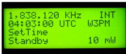
Depress and hold the “Clock Set” pushbutton while resetting the Mega 2650 to enter the time set routine. While holding the “Clock Set” button, depress the “Hours” and “Minutes” pushbuttons to set the time. Releasing the “Clock Set” pushbutton will start the clock.
