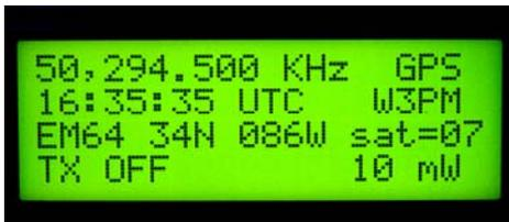
NMEA GPS is the preferred method of timing. It is available worldwide and will provide automatic “on-the-fly” calculation of the grid square location. It will also provide a LCD display of latitude and longitude and the number of satellites within range.
