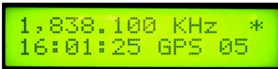
The transmitter may be put into a standby mode by depressing the Transmit Inhibit pushbutton. Depress again for normal operation. An asterisk will appear in the upper right-hand corner of the display when in standby. The GPS or WWVB receiver will remain on for time updates during standby periods.
