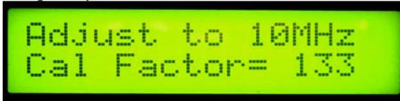
The DDS-60 requires frequency calibration unless you are using a GPS disciplined oscillator or other high precision frequency source for the 30 MHz oscillator.
